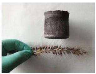
If collision accident happened or other accident which leads to leakage pollution happened, Ningbo-Zhoushan port can use the "Carbon sponge" to absorbing liquid contaminants fastly.
