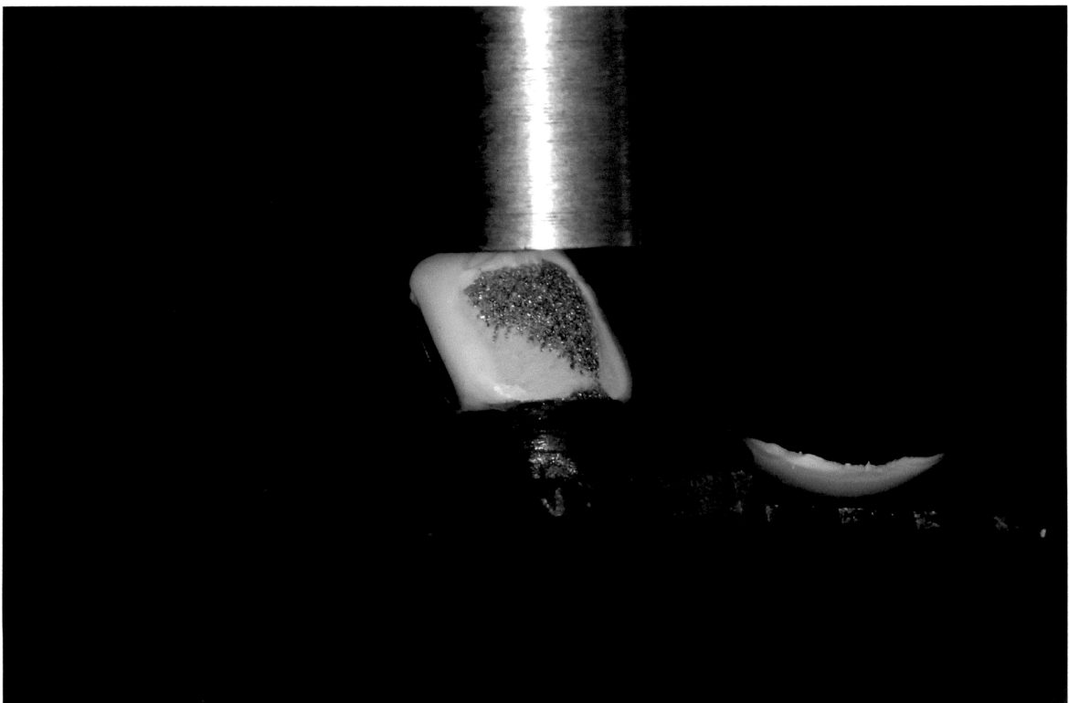
Figure 3. Typical veneer fracture.
