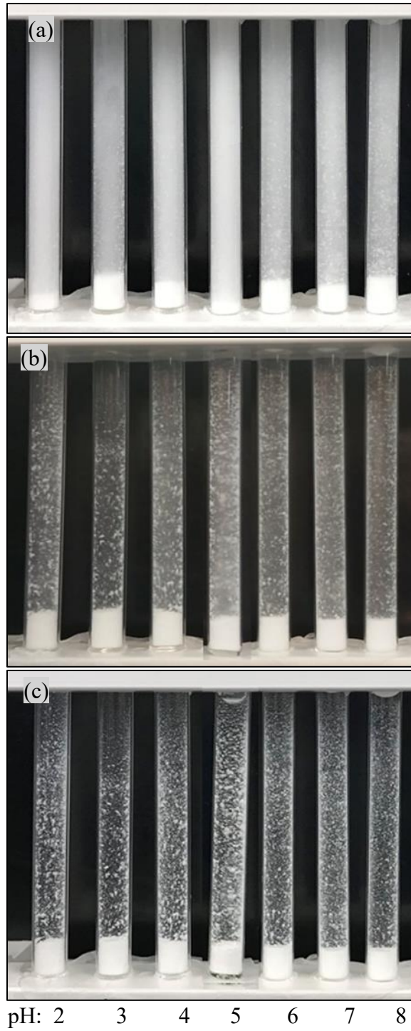
Figure 3.2. Gravity settling experiment results of BC-SSQ microparticles ( \phi_{\text{micro}} = 10^{-2} ) without nanoparticles (a) at start (b) after 2 hours (c) after 6 hours at different pH values of 2 to 8.
