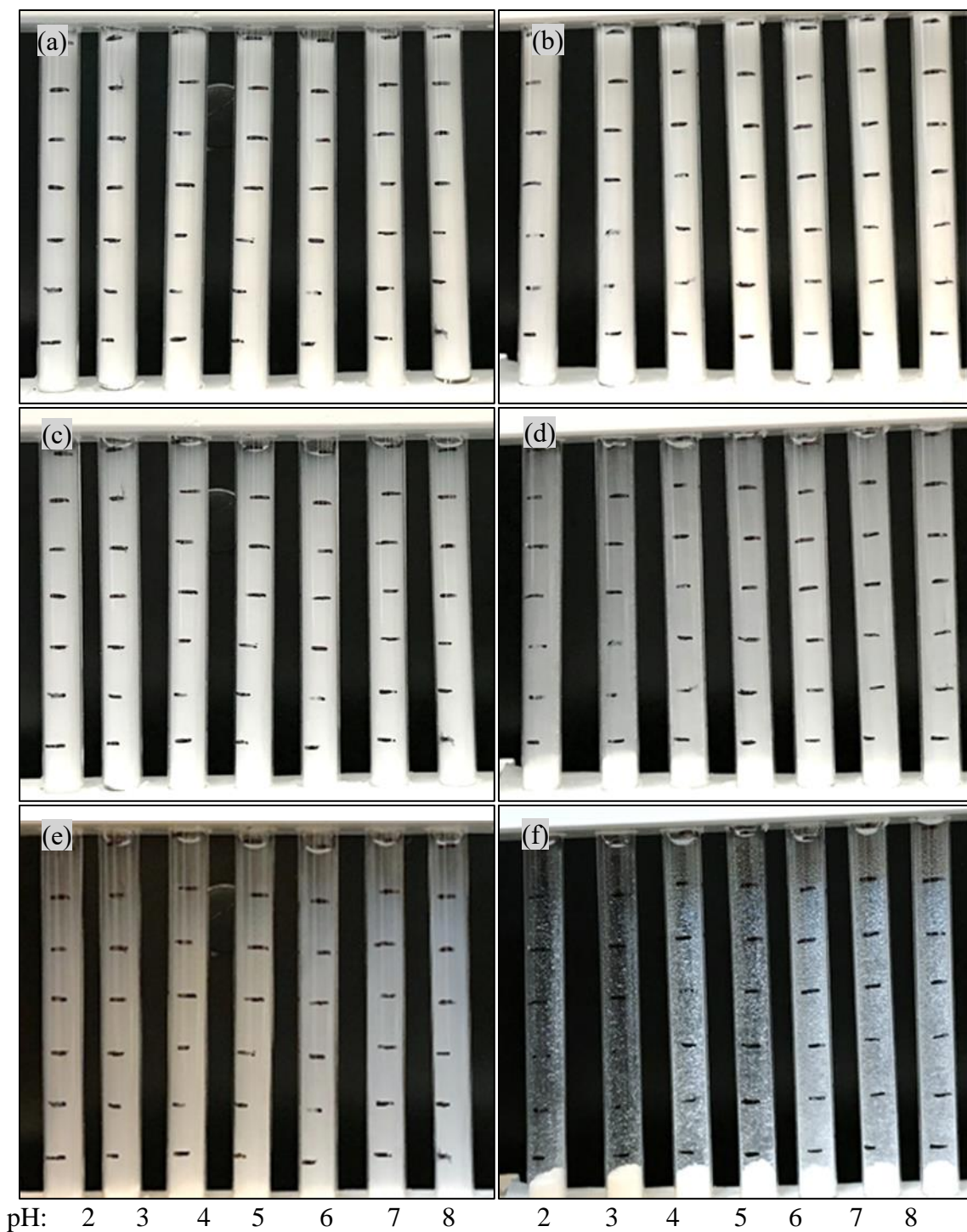
Figure 3.3. Gravity settling experiment results of binary systems of BC-SSQ microparticles ( \phi_{\text{micro}} = 10^{-2} ) with \text{SiO}_2 nanoparticles at (a) \phi_{\text{nano}} = 10^{-4} at start (b) \phi_{\text{nano}} = 10^{-3} at start (c) \phi_{\text{nano}} = 10^{-4} after 2 hours (d) \phi_{\text{nano}} = 10^{-3} after 2 hours (e) \phi_{\text{nano}} = 10^{-4} after 6 hours (f) \phi_{\text{nano}} = 10^{-3} after 6 hours at different pH values of 2 to 8.
