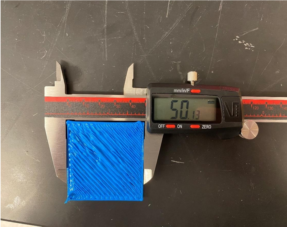
Figure 4.14 Measuring Dimensions of Sample Print Using Digital Calipers
