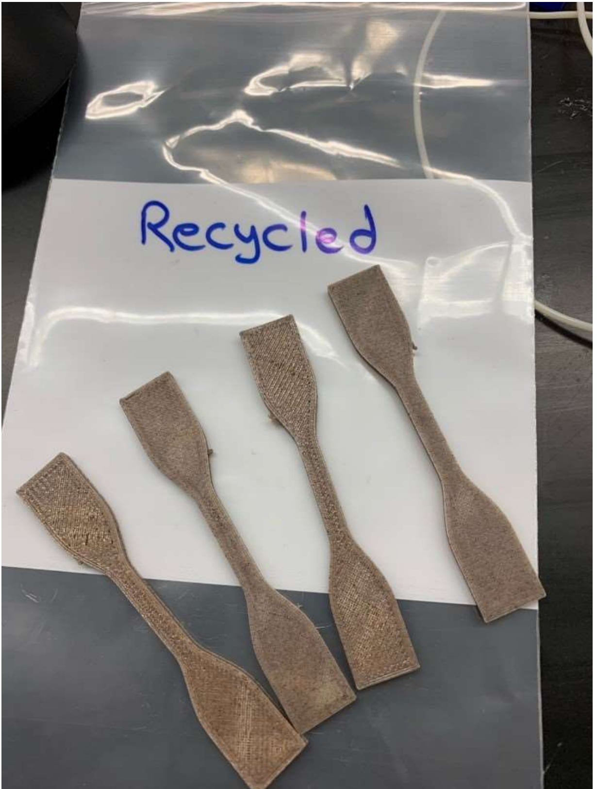
Figure 25. 3D printed parts with recycled Soybean fibers filled HYTREL
