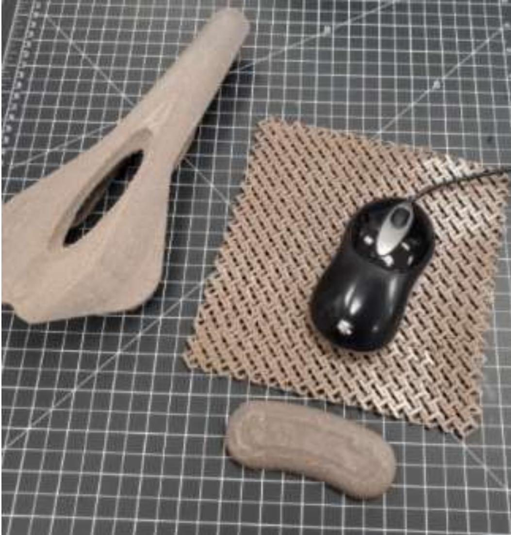
Figure 29. 3D printed parts with Soybean fibers filled HYTREL by somerset community college
