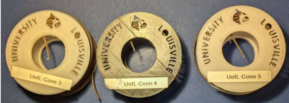
Figure 16. Soyhull fibers reinforced polymer composite filament spools with different fiber loadings (10% & 20%)
