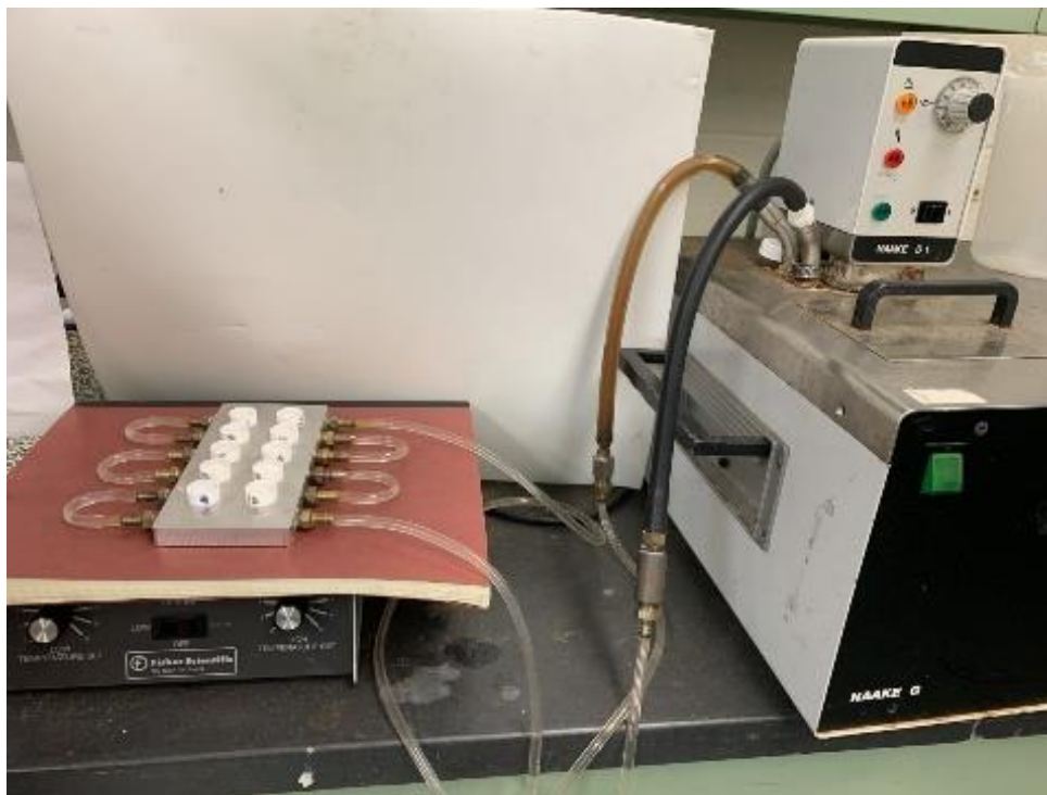
Figure 3.2(5). Heat Source. The investigators (Sledge and Borchman) designed the heating apparatus, and it was created in-house at the University of Louisville. The water enters into the metal plate from the heat bath and circles around the samples. The temperature is controlled from the heat bath and measured with a thermometer.
