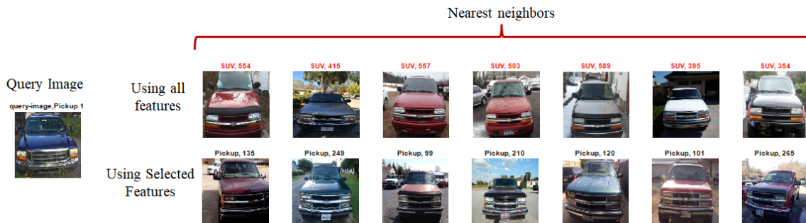
Figure 5.10: The nearest neighbors of a query-image-3. The first row shows the nearest neighbors using all the features. The second row shows the nearest neighbors considering only the learned features of each training samples in distance calculation. The class label of each image is displayed above the image. Nearest images from the incorrect class are indicated with red labels.
