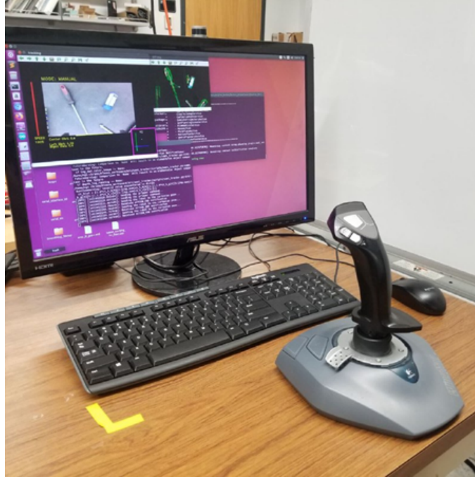
Figure 4.17: The base station from which the operator controls the robot during the experiments, showcasing the monitor with UI and the joystick. In these experiments, the user is not permitted to observe the robot workspace directly, only receiving visual feedback through the UI. In the image, the whiteboard to the right blocks the view of the robot.
