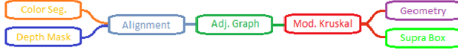
Figure 4.6: Method for joining regions in the depth and color spaces into coherent graspable surfaces
