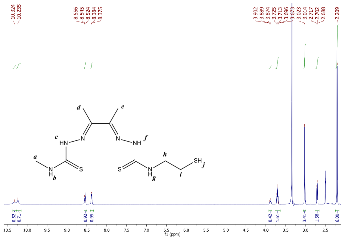
Figure A.3. 1 H NMR of Diacetyl-N-methyl-N'-(2-mercaptoethyl)-bis(thiosemicarbazone) ( 4 ). \delta (ppm) = 10.32 (br. s, 1H c ); 10.23 (br. s, 1H f ); 8.54 (t, J = 5.5 Hz, 1H g ); 8.38 (q, J = 4.5 Hz, 1H b ); 3.89 (br. s, 1H j ); 3.70 (q, J = 8.5 Hz, 2H i ); 3.34 (s, H 2 O); 3.01 (d, J = 4.5 Hz, 3H a ); 2.70 (t, J = 7.5 Hz, 2H h ); 2.50 (m, DMSO); 2.21 (s, 3H d ); 2.20 (s, 3H e ); 2.07 (s, MeCN)
