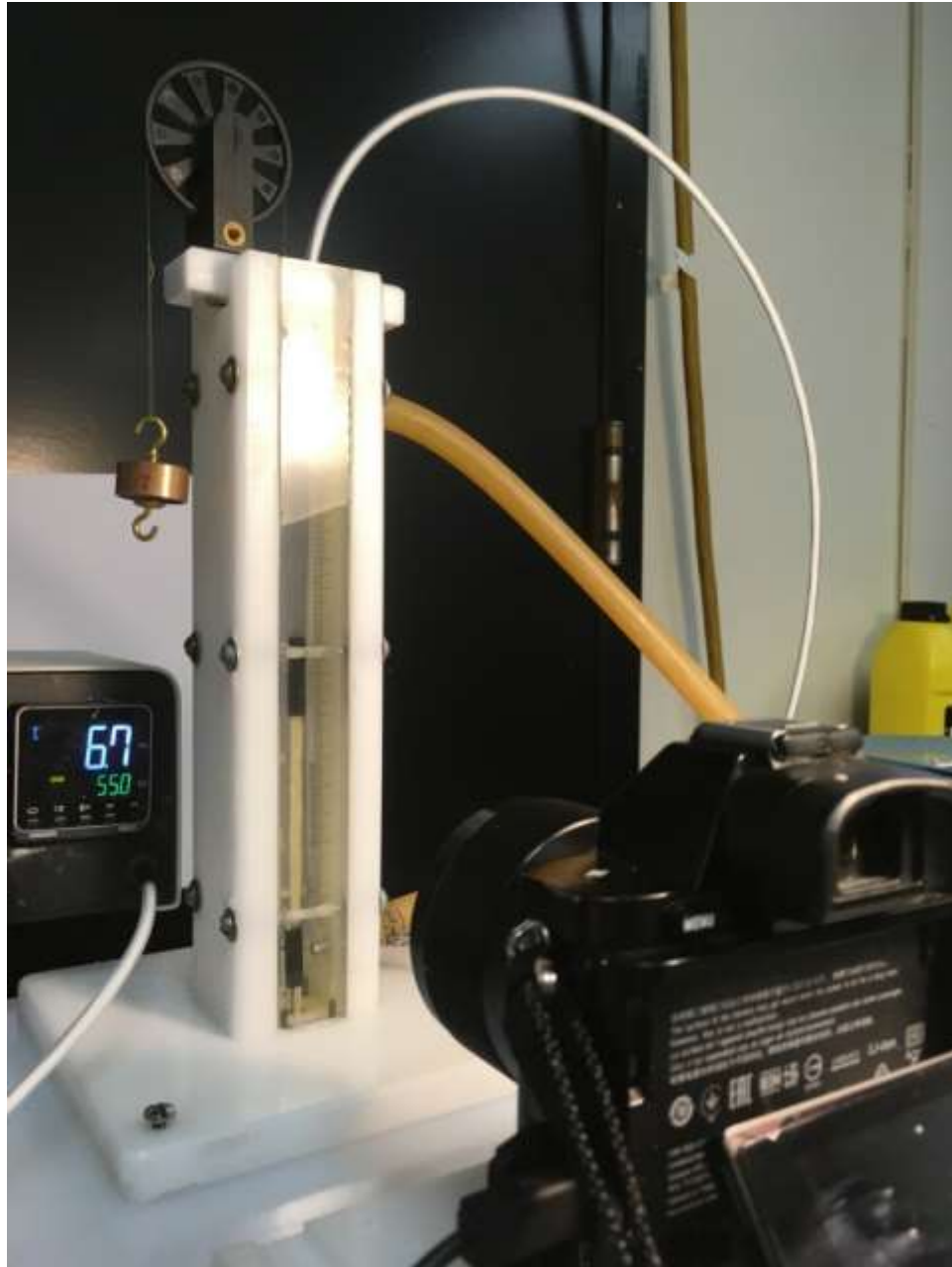
Figure 4.2. The thermomechanical setup. The fiber length, temperature and masses are recorded by the camera.
