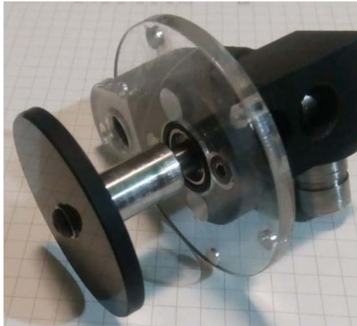
Figure 8: SAV plunger and shuttle
