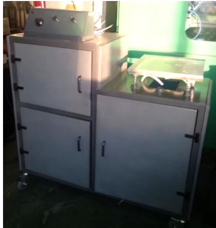
Figure 12: Manufactured casting unit
