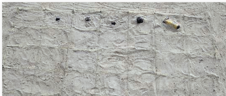
Figure 9. Submunition targets and example night-time anomalies from Night 3 at 23:00. Anomalies and targets are presented approximately to scale. Burial depths for TIR anomalies above are as follow: M42: 1.0 cm, M77: 1.0 cm, BLU-63: 1.0 cm, BLU-61: 0.7 cm, BLU-97: 1.3 cm.
