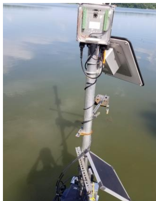
Figure 4.2: Image of the weather station affixed to a cooperating landowner's dock.
