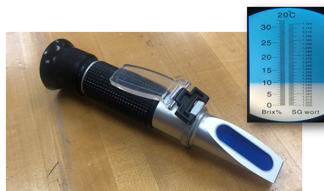
Figure 2. Brix meter used to determine sweetness on the brix scale
