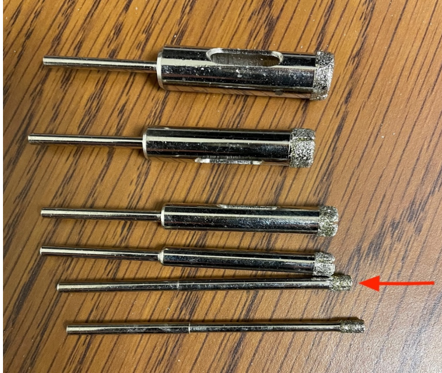
Figure 2: Set of diamond core bits. Arrow indicating the selected size used in the coring method.
