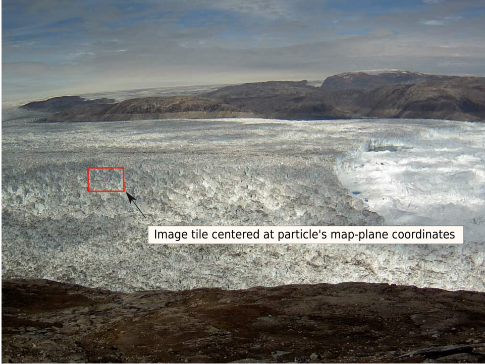
Figure 6: For a given point in map-plane coordinates, the image sub-sampling function extracts a tile centered around the point from the camera’s perspective
