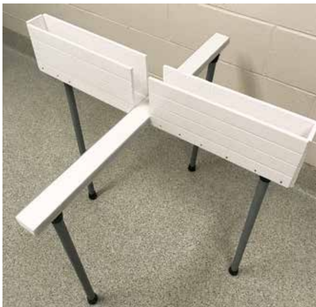
Figure 4. The EPM assess rodent anxiogenic behavior based on their natural aversion of open spaces. Photo courtesy of Pitychoutis Laboratory, 2019.
