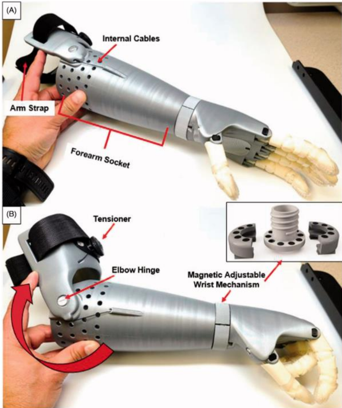
Figure 3. 3 D-printed elbow-driven prostheses. (A). shows the device in the open position. Elastic cords placed inside the dorsal aspect of the fingers provide passive finger extension. (B). Finger flexion is activated through 10–20° of elbow flexion of the residual functional joint. The red arrow shows the direction of elbow flexion to close the fingers and produce a functional grasp. The wrist can be manually adjusted. No harnessing is required to suspend the prosthesis.
