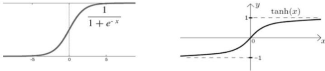
Figure 5. Activation functions. (1) the left curve is a sigmoid function curve. (2) the right curve is a tanh function curve [35].
