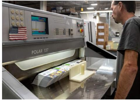
A College Press worker cuts papers. The guillotine-like machine cuts several blocks of paper at a time for efficiency. There were several stacks of paper on the other side of the machine.
