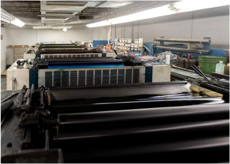
The coloring presses process sheets of paper. These six presses can run 10,000 sheets of paper per hour.
