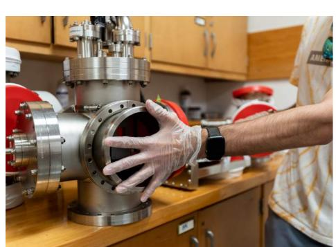
Arian Dovald demonstrates where a gasket will connect to a tube containing a faraday cup, a sensor used to monitor what is happening within the beamline. Due to the metal tubes being very sensitive, people operating the machine must wear gloves to prevent dust or skin oils from touching the inner portions of the tubes.
