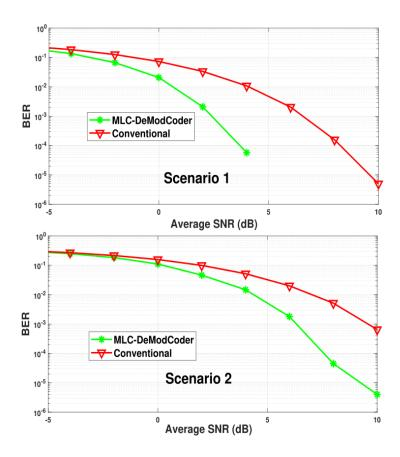
Figure 9. BER vs. Average SNR (dB) for Proposed and Baseline Scheme 1 for Scenario 1 and Scenario 2.
