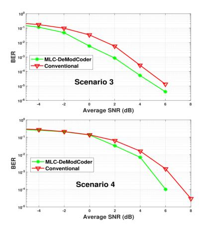
Figure 10. BER vs. Average SNR (dB) for Proposed and Baseline Scheme 1 for Scenario 3 and Scenario 4.
