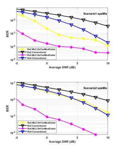
Figure 16. BER vs. Average SNR (dB) for The Proposed and Baseline Scheme for Scenario 1 and Scenario 2 under  $\epsilon$ -Mixture Noise for Rx2 and Rx4.
