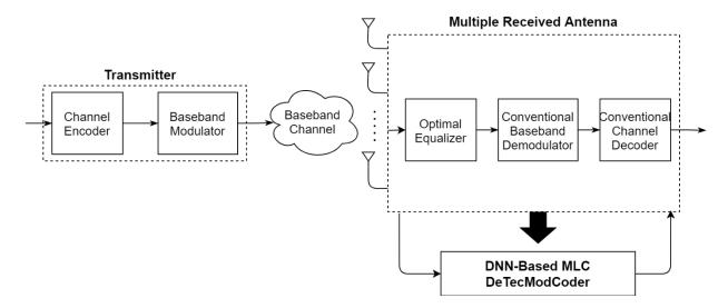
Figure 12. Multiple Receiver Communication Links with Conventional vs. AI-Based Receiver Processing.
