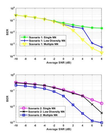
Figure 14. BER vs. Average SNR (dB) for Scenario 1 and Scenario 2 Using Single, Low Diversity and Multiple NNs for Rx2.
