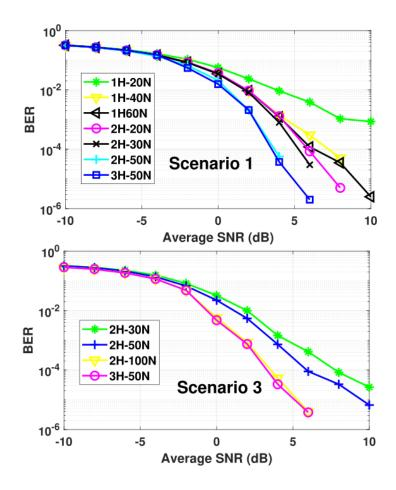
Figure 7. BER vs. Average SNR (dB) for DNN-Based MLC DeModCoder for Scenario 1 and Scenario 3.
