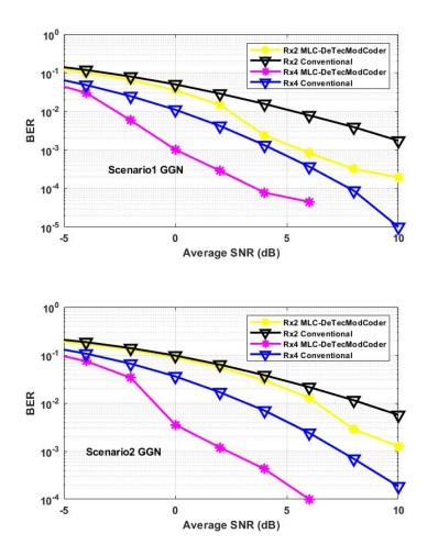
Figure 17. BER vs. Average SNR (dB) for The Proposed and Baseline Scheme for Scenario 1 and Scenario 2 under GGN for Rx2 and Rx4.
