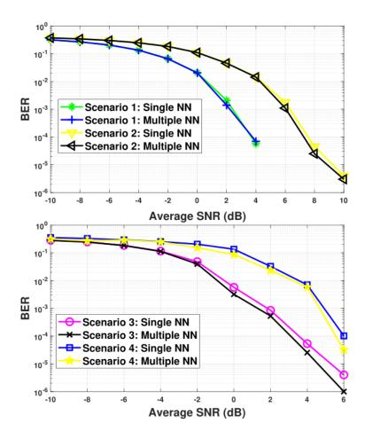
Figure 8. BER vs. Average SNR (dB) for DNN-Based MLC DeModCoder Using Single and Multiple NNs.
