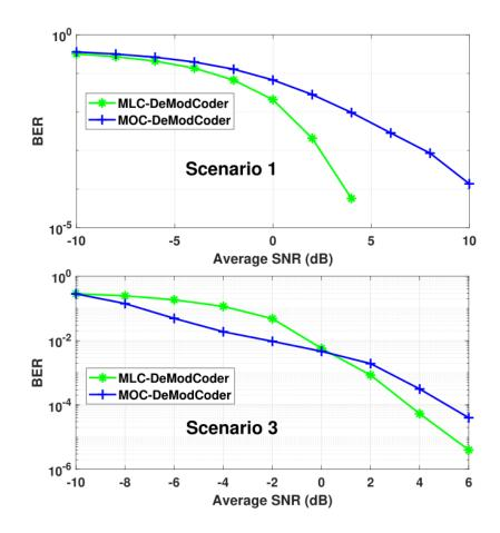
Figure 11. BER vs. Average SNR (dB) for Proposed and Baseline Scheme 2 for Scenario 1 and Scenario 3.
