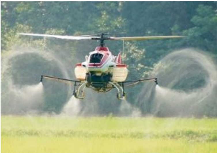
Figure 2.5 Agriculture Drone is spraying pesticides on crops.
