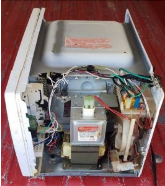
Figure 11.3: Inside of ordinary kitchen microwave oven
