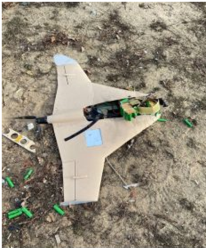
Figure 6.10: The Wreckage of Another Russian KUB-BLA Loitering Munition.
