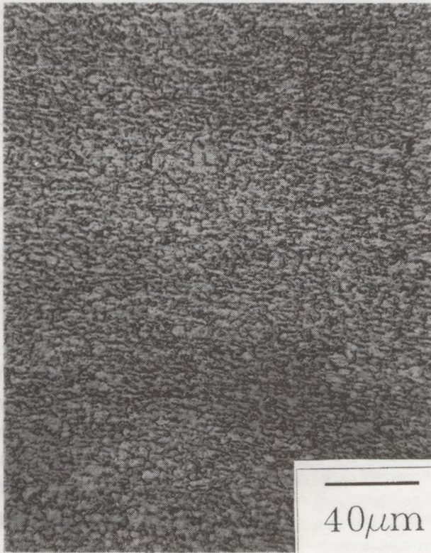
FIGURE 4 Optical Microstructures of the Parent Metal (top left), Heat-Affected Zone (top right), and Fusion Zones (bottom right and left), Longitudinal Views
