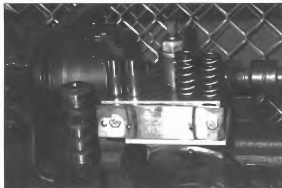
FIGURE 3 Test Apparatus: Test Equipment Mounted in Lathe (Front View)
