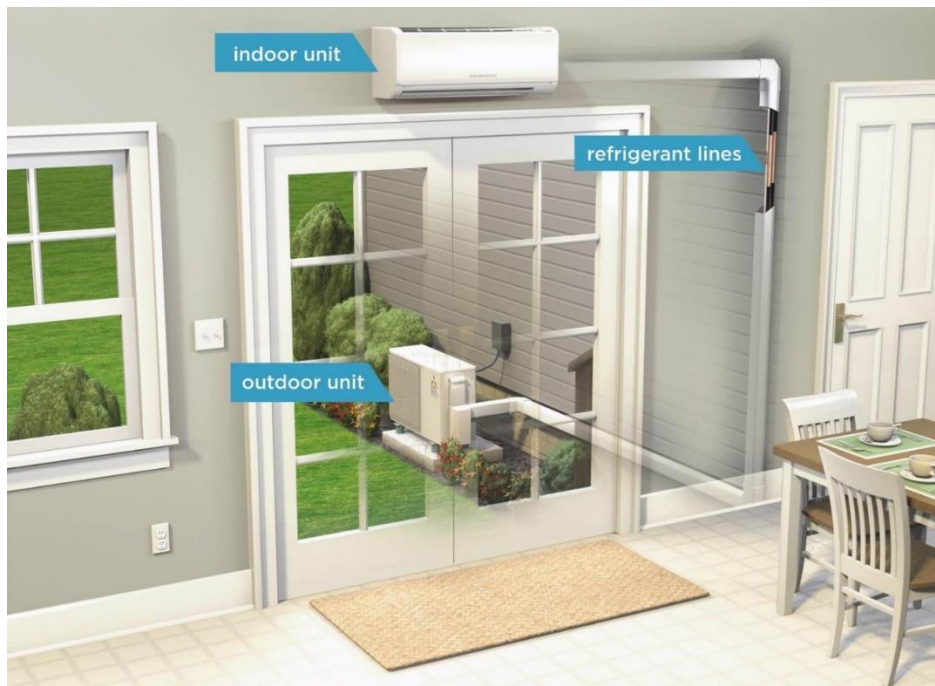
Figure 17: Mini-split Heat Pump (26)
