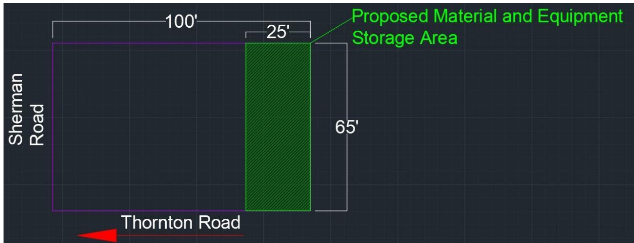
Figure 4: Material Delivery and Storage Plan
