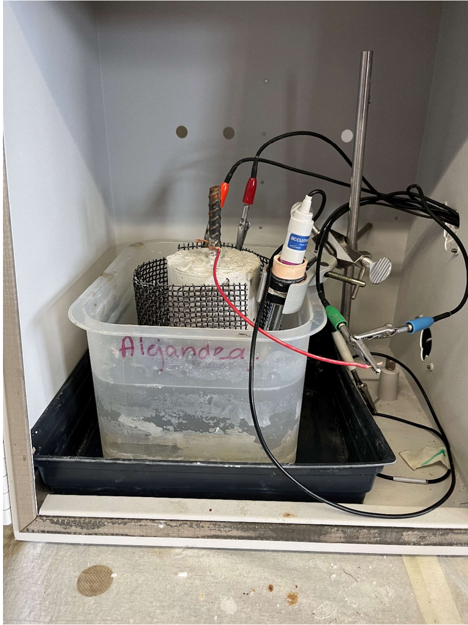
Figure 1: Photograph of the reference cell set-up that was used to gather OCP, EIS, and CPP data.
