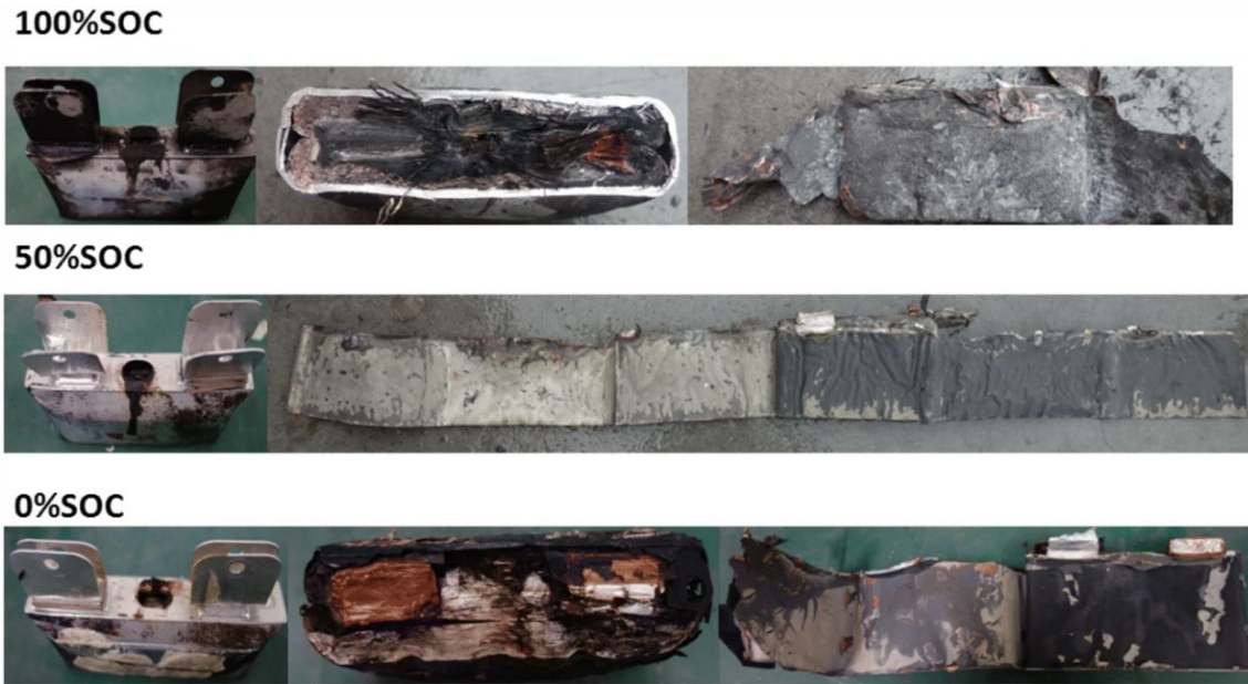
Figure 1: Result of Thermal Runaway for Various States of Charge as shown in “Thermal Behavior and Failure Mechanism of Large Format Lithium-Ion Battery.”
