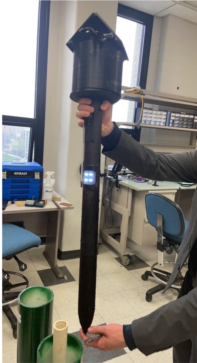
Fig 18: Completed Design With ABS and PLA+ Plastic Housing
