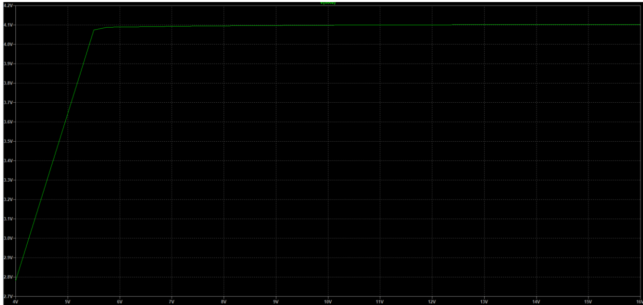
Fig. 26: Charging Circuit Output
