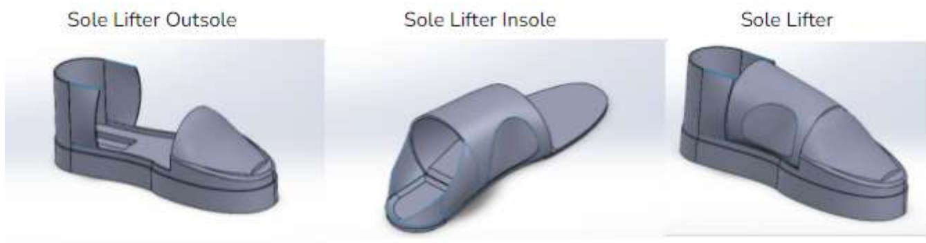
Figure E: SolidWorks 3D Models of Sole Lifter Design to verify feasibility; Outsole on left, Insole mechanism in center, combined SolidWorks models on right
