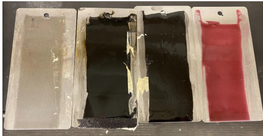
Figure 7. From left to right is the synthesized coating, HEUCODUR 953, HEUCODUR 9-100, Clariant Black CLN.
