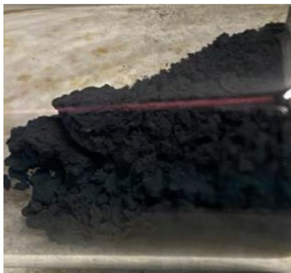
Figure 1. \text{Ca}_2\text{Mn}_{0.65}\text{Ti}_{0.15}\text{Zn}_{0.20}\text{O}_{3.80} synthesized pigment.
