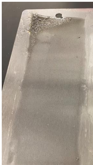
Figure 6. This panel is coated with the synthesized coating with 6.48 weight percent pigment.
