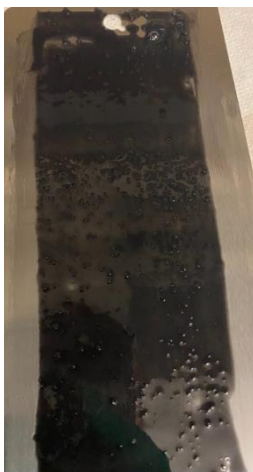
Figure 5. This panel is coated with the synthesized coating with 25.91 weight percent pigment.
