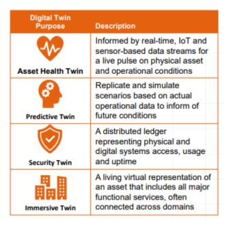
**Figure 11:** The figure displays the diagram explaining the different purposes of digital twins. This diagram was used in a 2022 presentation by James Cooper of Arcadis [6].
