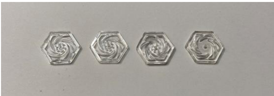
Figure 20: Photo of the results from the layer exposure time tests for the clear plant-based Anycubic resin. The 2 second sample did not stick to the build plate and is not pictured. The 6, 10, 14, and 18 second samples are shown from left to right.
