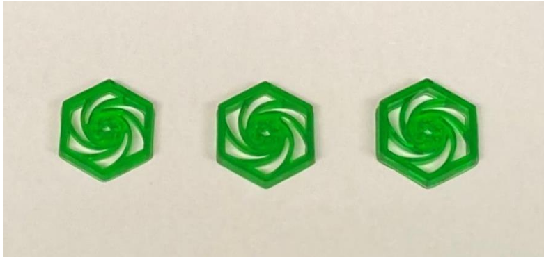
Figure 7: Photo of the results from the base exposure time tests for the provided green Anycubic resin. The 20 second sample did not stick to the plate and is therefore not pictured. The 40, 60, and 80 second samples are shown from left to right.
