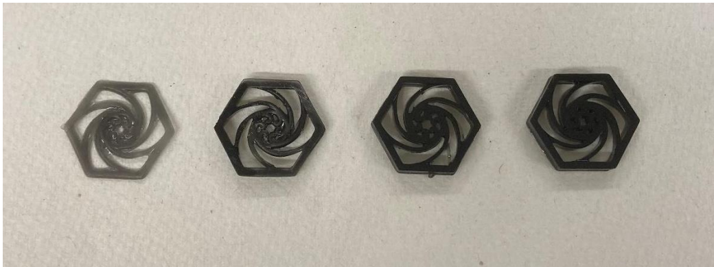
Figure 14: Photo of the results from the layer exposure time tests for the F69 TPU-like resin. The 2 and 6 second samples did not stick to the build plate. The 6 second sample is pictured on the left as an example of a failed print, and the result was salvaged from the bottom of the resin vat. The subsequent 10, 14, and 18 second samples are shown from left to right.
