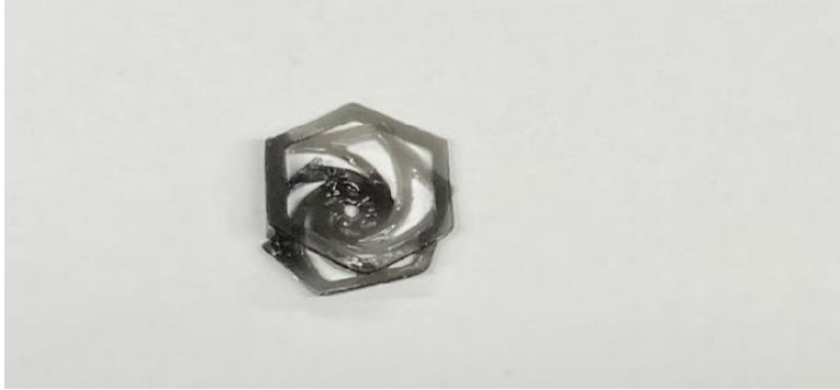
Figure 15: Photo of the results from the base exposure time tests for the Wanhao flexible rubber resin. The sample shown is the 80 second sample, and the 20, 40, and 60 second samples did not stick. The sample still was still very easy to remove, so each of the base exposure tests was considered failed.
