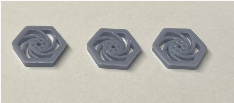
Figure 12: Photo of the results from the layer exposure time tests for the gray ELEGOO ABS-like resin. The 2 and 6 second samples did not stick to build plate and are not pictured. The 10, 14, and 18 second samples are shown from left to right.
