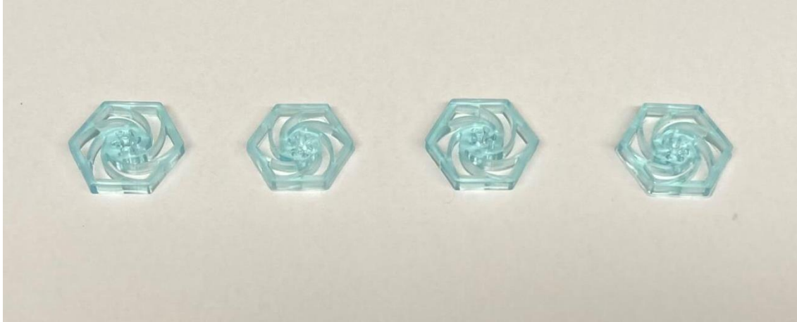
Figure 9: Photo of the results from the base exposure time tests for the blue ELEGOO Water-Washing resin. All prints are stuck to the plate, and the 20, 40, 60, and 80 second test samples are shown from right to left.
