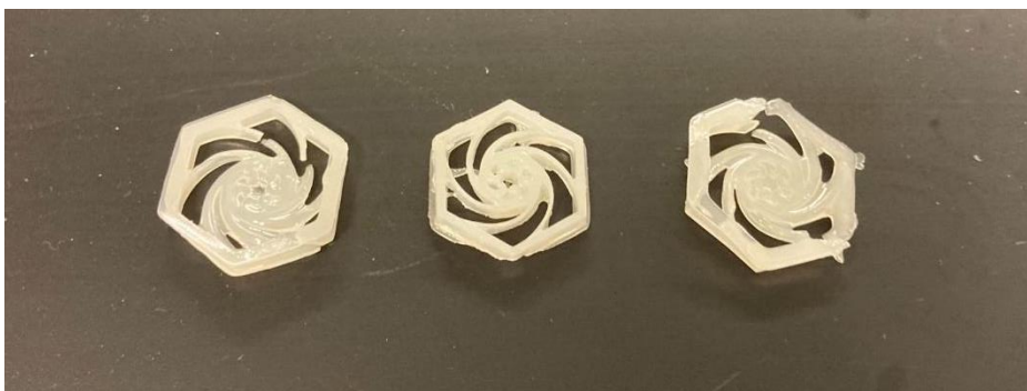
Figure 17: Photo of the results from the base exposure time tests for the iFun toughness resin. While all samples have significant defects, the 40, 60, and 80 second samples are shown from left to right.
