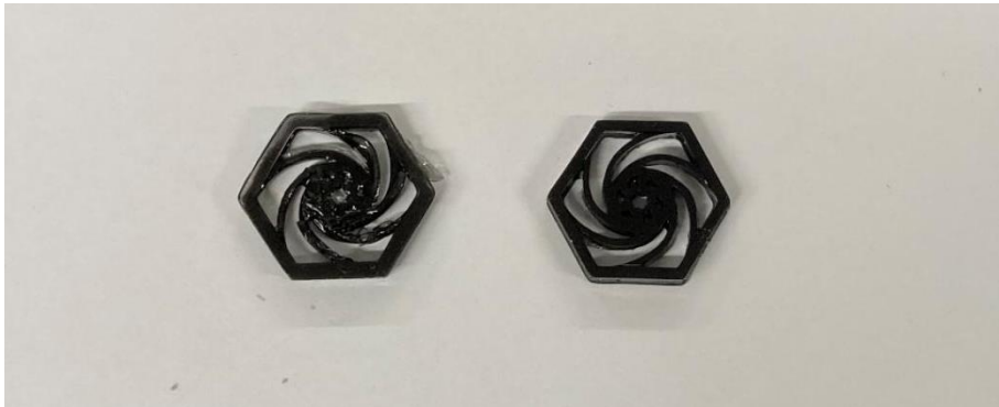
Figure 16: Photo of the results from the layer exposure time tests for the Wanhao flexible rubber resin. The 2, 6, and 10 second samples did not stick to the build plate and are not pictured. The 14 and 18 second samples are shown, respectively. The 14 second sample had significant layer separation.
