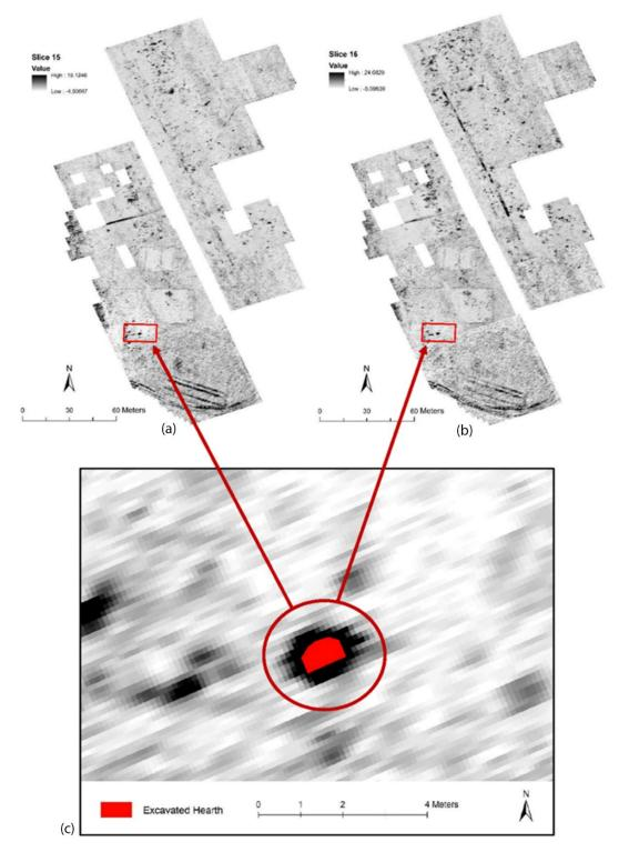
**Figure 4.** GPR slice mosaics showing the hearth excavation area: (a) Slice 15; (b) Slice 16; (c) Close-up of anomaly in Slice 15 with the red polygon representing the excavated hearth extent recorded by the Real-Time Kinematic (RTK) Global Navigation Satellite Systems (GNSS). GPR slice resolution is  $0.125 \times 0.125$  m.
