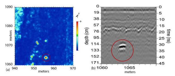
**Figure 3.** (a) Horizontal GPR Slice 15 of Grid C13 showing an excavated Archaic hearth at 1.02 m below surface (BS); (b) A portion of Radargram 33 showing the hearth's reflection pattern. Smaller hyperbolas representing multiple stacks of fire-cracked rock can be seen below the large flat hyperbola that represents the circular hearth as a whole.
