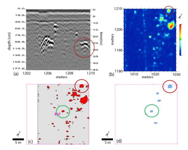
**Figure 6.** Four views of a probable Archaic hearth (circled in red) in Grid E17 extracted by the semi-automated OBIA model: (a) The reflection pattern in a portion of Radargram 44; (b) GPR Slice 14; (c) Map of objects extracted by global threshold segmentation; (d) Map of objects remaining after manual elimination of noise. Another probable hearth (circled in green) was identified and confirmed at a depth of 1.02 m BS during the auger testing.
