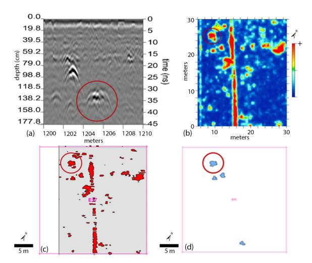
**Figure 8.** Four views of a probable hearth (circled in red) in Grid E17, which was confirmed by FCR in the auger at 1.18 m BS: (a) Reflection pattern in a portion of Radargram 8; (b) GPR Slice 16, where linear features from a known electrical line are also clearly visible; (c) Map of objects after global threshold segmentation; (d) Map of objects remaining after the OBIA and manual elimination.
