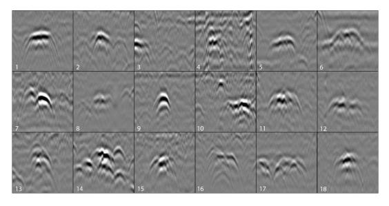
**Figure 9.** Radargrams showing probable Archaic hearth reflection patterns, which correspond to test results shown in Table 3.
