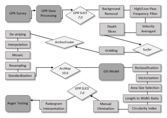
**Figure 2.** Workflow chart showing steps of Ground-Penetrating Radar (GPR) data processing and object-based image analysis (OBIA) GIS model.
