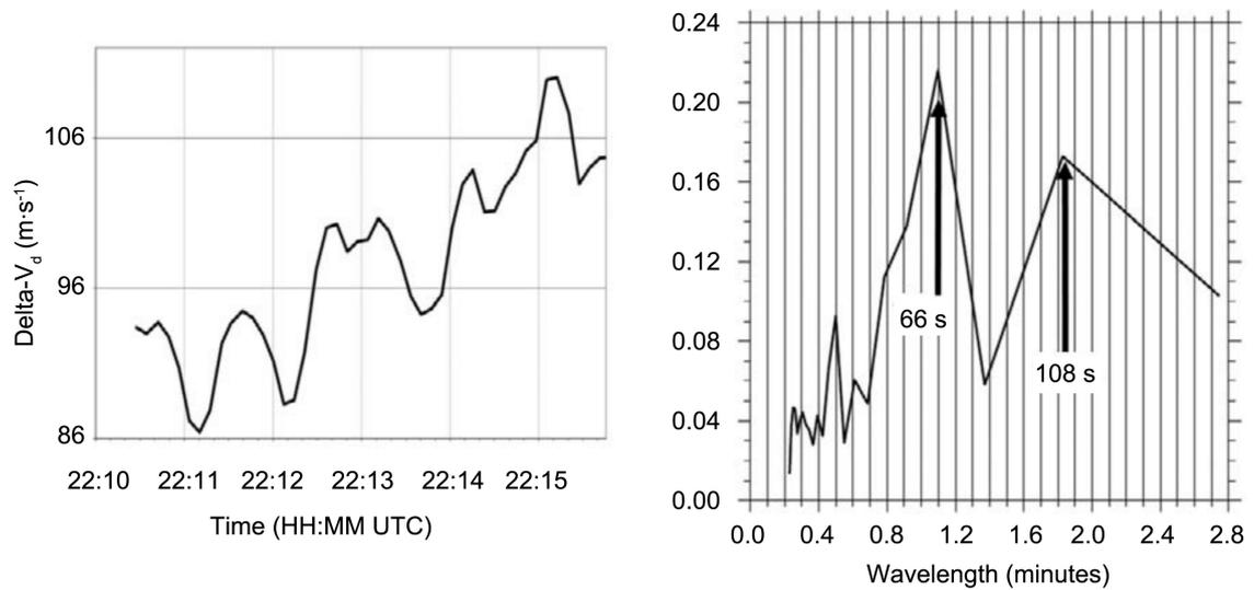
**Figure 5.** Time series of maximum gate-to-gate shear,  $\Delta V$ , consistent with energy being pumped into the tornado in discrete pulses, possibly from roll-up vortices within a vortex sheet (left); FFT of  $\Delta V$  with peak energy at 66 seconds and 108 seconds (right), suggestive of rotating asymmetry in the vortex; © AMS, [53].
