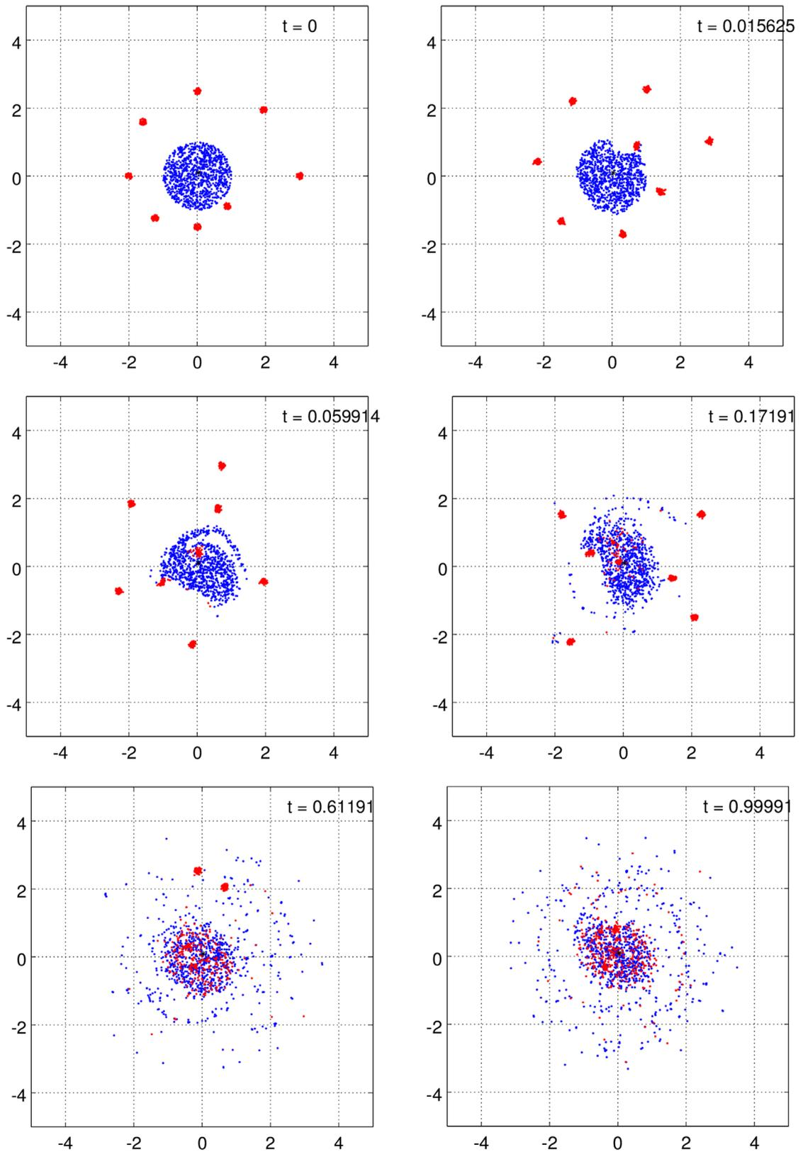
**Figure 3.** An illustration of the dynamics of a vortex gas using point vortices in two dimensions. Smaller vortices (red) around a larger vortex (blue) are being absorbed and dispersed in the surrounding flow. Non-dimensional lengths and time are used.
