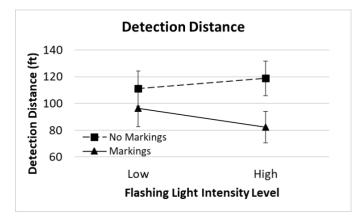
Figure 10 - Average (+/- standard error of the mean) detection distances for each combination of intensity level and the presence of reflective markings
