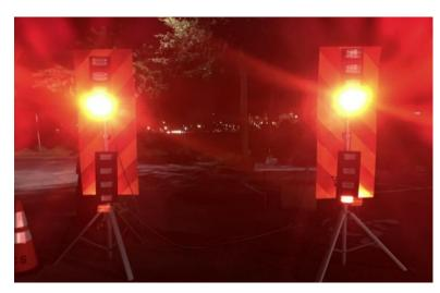
Figure 3 - Mounting configuration for the flashing emergency lights used in the study; also shown are reflective marking panels behind each set of lights
