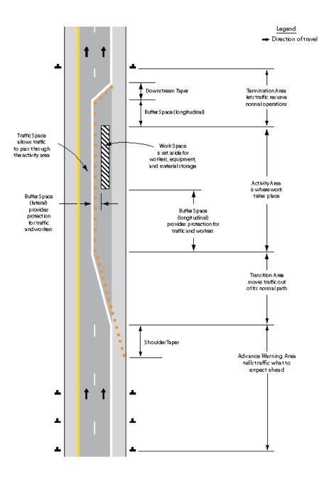
Figure 4 - Diagram of cone taper for incident management response (U.S. DOT and FHWA, 2021)
