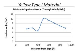
Figure 11 - Minimum luminances of yellow ASTM Type I (a)
