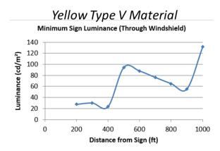
Figure 12 - Type V (b) materials as a passenger vehicle with low-beam headlights approaches
