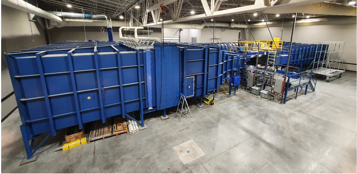
Figure 2.1 Embry-Riddle Aeronautical University's closed-return wind tunnel facility located at the MicaPlex Research Park.
