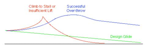
Figure 10: Possible glider paths. (does not show possibility of loop-de-loop).
