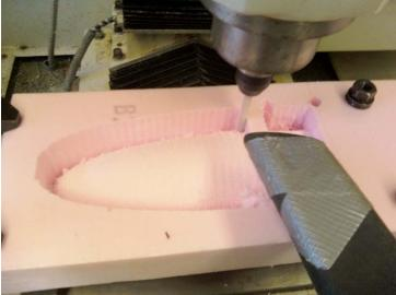
Figure 7: CNC Mill Machining Half of the Fuselage.
