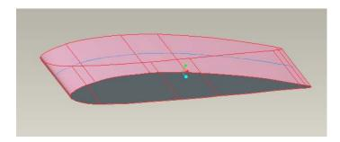
Figure 5: Surface profile used by CNC milling machine.
