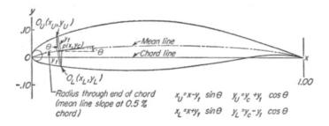
Figure 1: Visual definition of four digit airfoil geometry.<sup>26</sup>
