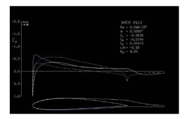
**Figure 2:** NACA 2412 XFOIL PRESSURE DISTRIBUTION ( $\alpha = 0$ )
