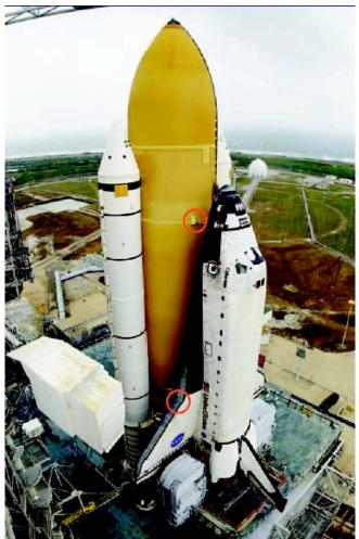
Figure 5: Picture of Columbia shuttle stack with locations of foam and impact marked.
