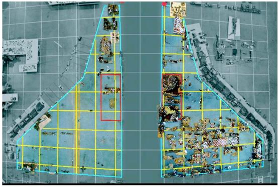
Lower Left wing debris Figure 6: Top view of recovered debris from Columbia's wings.<sup>1</sup>
