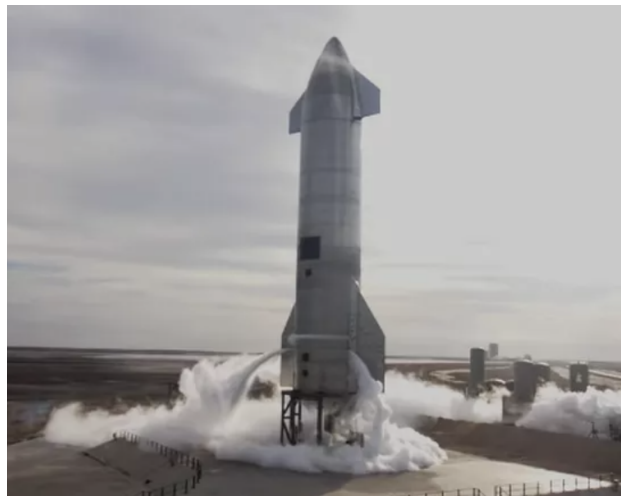
Figure 2.3: Starship SN15 Body [12]. Note the wide non-symmetrical cross-section of the vehicle which makes it difficult to control a gravity flip turn in the upper atmosphere
