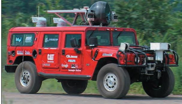
CARNEGIE MELLON RACE TEAM'S "H1lander" turned out to be a successful contender for the 2005 Grand Challenge. The 1999 Hummer H1, donated by AM General, uses an electronic CANbus, a 6.5-liter factory turbo-charged diesel engine, traction control and locking differentials.
