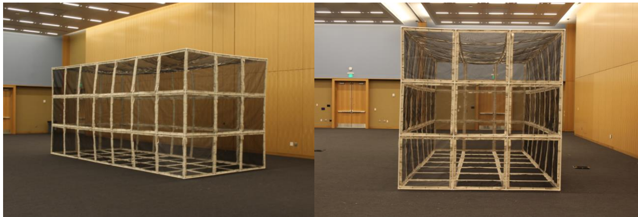
Figure 9: Fully constructed drone cage at its maximum size.
