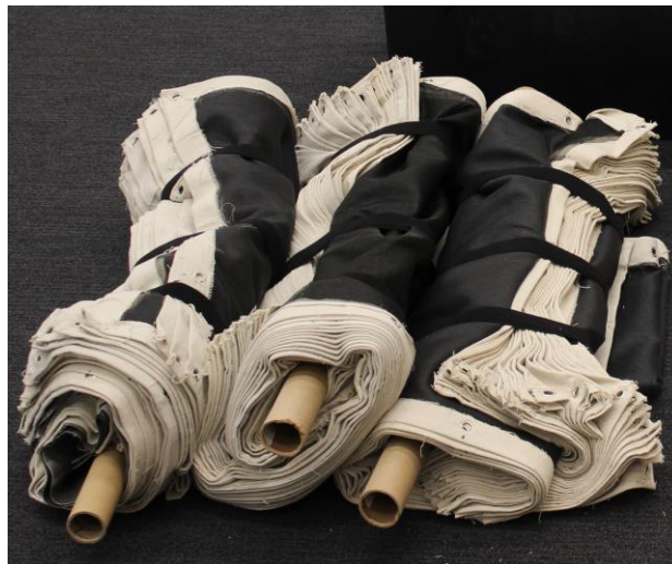
Figure 6: Rolls of fabricated netting with canvas-cloth lined edges and grommets.
