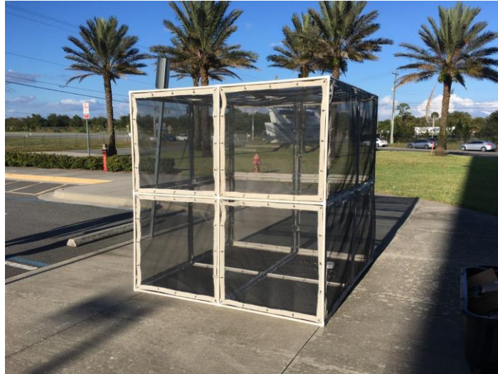
Figure 8: A 2m x 2m x 2m constructed model of the drone cage.
