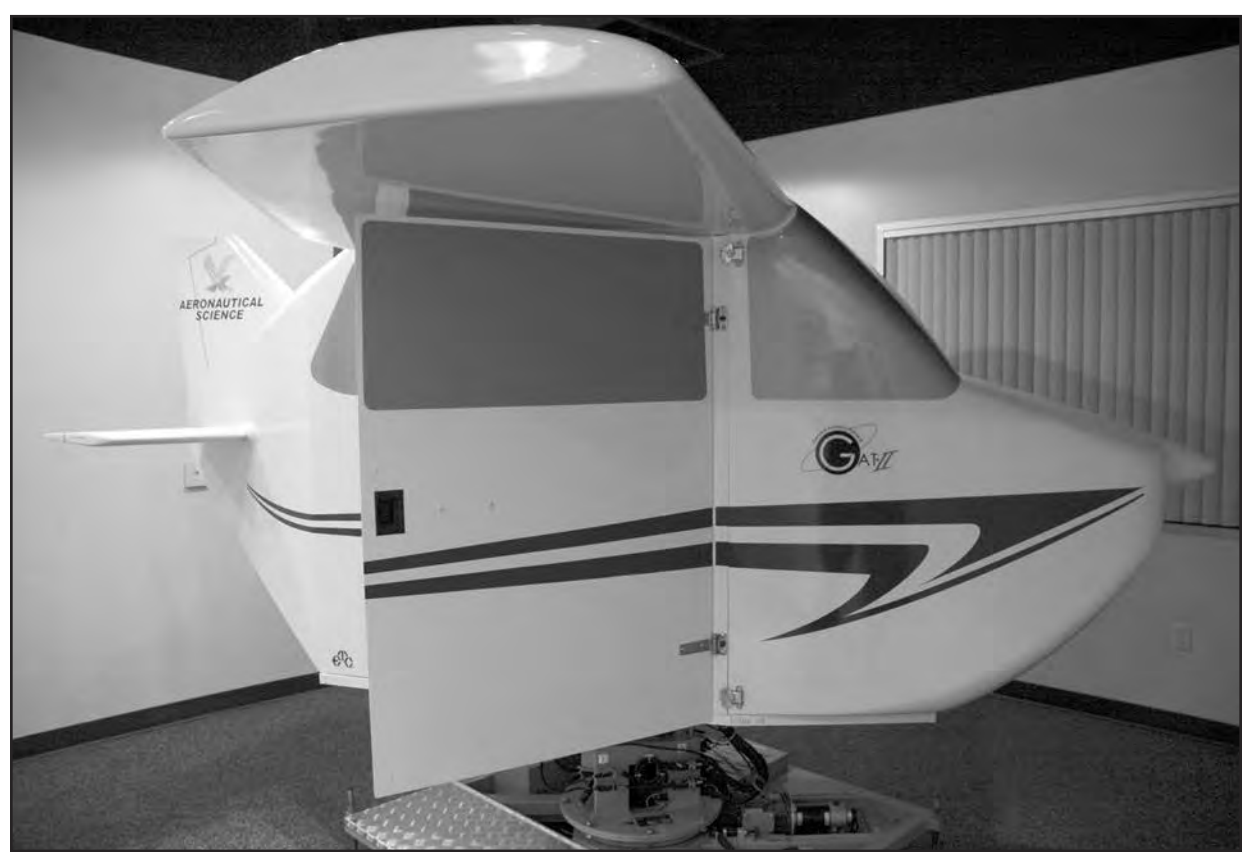
THE GAT II TRAINER simulates many of the common illusions that can cause pilots to lose control of their aircraft. To sign up for a free demo ride, visit the Flight Tutor Lab in the College of Aviation building.
