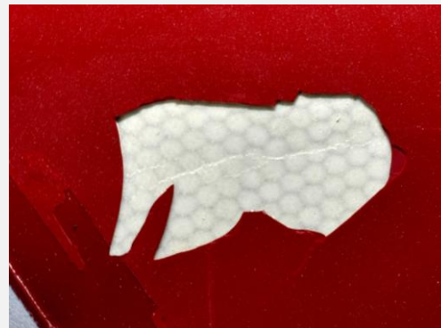
Damage on radome nose.
