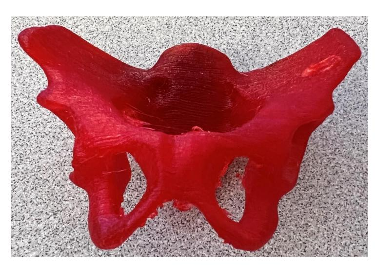
The printer the pelvis was printed on is the FlashForge Creator Max 2, however the team has recently concluded the purchase of an Ultimaker S5 printer to further expand their 3D printing capabilities. The pelvis was printed using SainSmart 95A Red TPU Filament.
