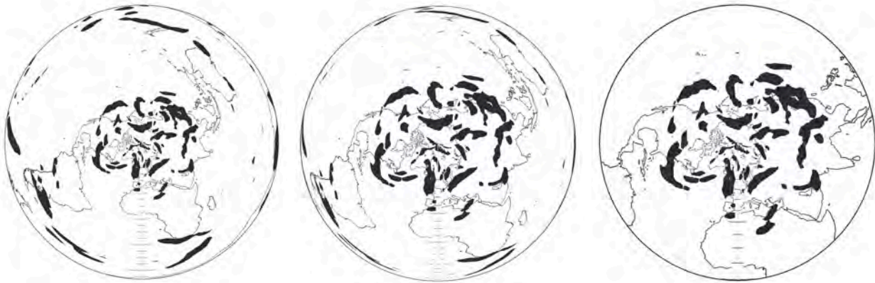
Figure 3.31. A comparison between azimuthal map projections with data: (left) azimuthal equidistant, (center) Lambert azimuthal equal-area and (right) stereographic which is conformal. Adapted from, Richter, Sassi et al. (2010).
