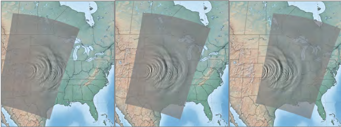
Figure 4.26. Simulated images of CO 2 BWT as seen by an imager on board a satellite with parameters: 725 km height, 7.5 km/s orbital velocity, 14.4° azimuth track, 2.67 s time between exposures, 512 cross-track pixels and 48.7° FOV. (left) track shifted by 500 km East. (center) original track through center of data. (right) track shifted by 500 km West.
