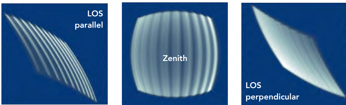
Figure 1.9. Zenith and off-zenith synthetic CCD images. (top) oblique view of the imager where LOS is parallel to the wavefronts and creates intensity enhancements. (middle) Zenith imaging contains little to no LOS effects. (bottom) oblique view of the imager where LOS is perpendicular to the wavefronts with significant filtering of the horizontal wavelength.
