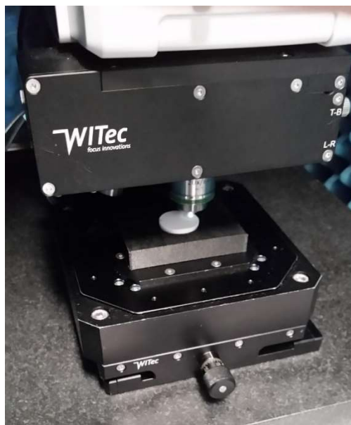
Fig. 2 Example of confocal Raman system setup
