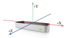
Fig. 3. Leap motion controller and coordinate system [13]
