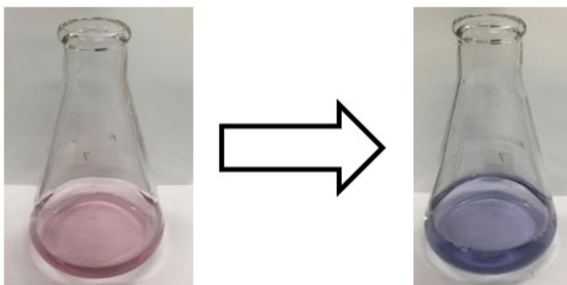
Figure 3.7: Color change as titration is performed carefully with the EDTA solution.
