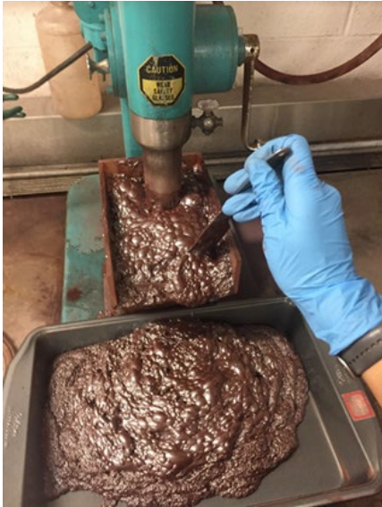
Figure 3.12: Flotation cell at Michigan Technological University laboratory.
