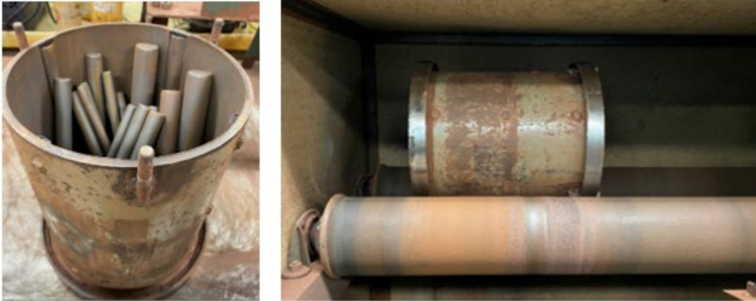
Figure 3.8: Grinding mill at Michigan Technological University laboratory
