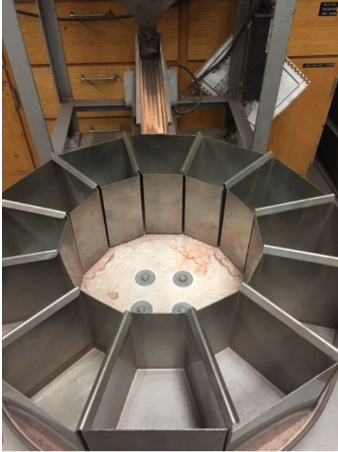
Figure 3.4: Rotary riffle splitter at the Michigan Technological University laboratory.
