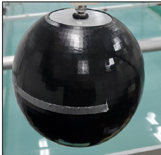
Figure 12: 3D Printed Spherical Buoy Test Artifact
